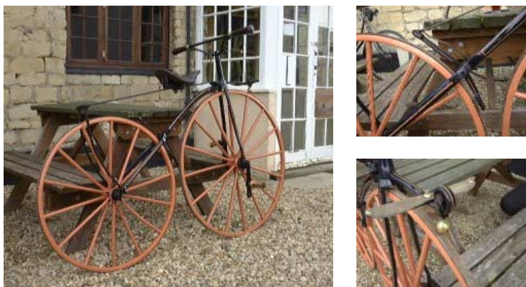
The oldest bike on display was this 'Boneshaker' from 1870/71, thought to have been built by Muire of Wolverhampton. It features a twist grip brake lever which activates a leather thong connected to the retardation device on the rear wheel. Note the foot rests above the front wheel, used mainly when going downhill. This is because the fixed pedal/wheel combination could reach considerable speeds!
